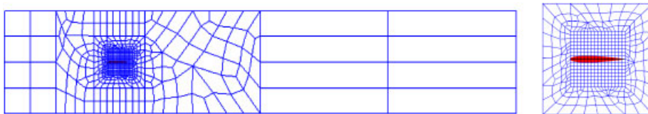
Figure 10. Coarse mesh for flow around a rotating NACA0012 airfoil (left is the global mesh, right is a local zoom covering the airfoil at Level = 1).
